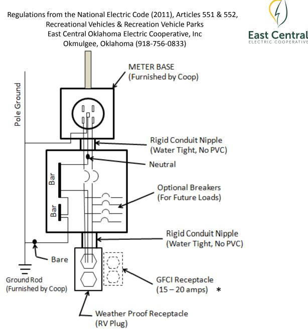
1.Article No. 552.10 (E) – Over current Protection Low-voltage circuit wiring shall.... Not be in excess of the ampacity of copper conductors, in accordance with Table 552.10 (E) (1) Note: Any service requiring 240 volts will be required to have a minimum of 50 amp breakers
