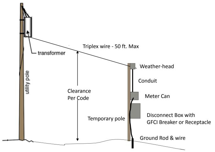
Note: Temporary pole, Weather-head, Meter Can, Ground rod & Disconnect Box – provided by member or designee. Pole to be installed securely – East Central Electric to inspect before terminating cables
