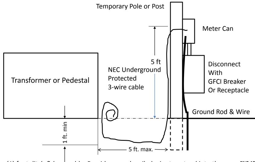
Dig one (1) foot ditch & bury cable. Provide enough coiled wire to extend into the padmount transformer
